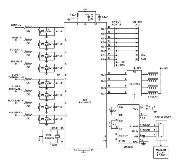
Fig. 5: Micro-Controller Pin Diagram
