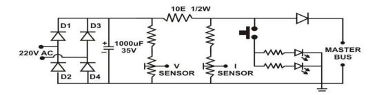
Fig.4 AC Sensing Card for Super Thermal & Nuclear Section
